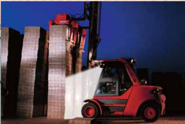
Lower reflector provides a broad and homogeneous ground illumination
