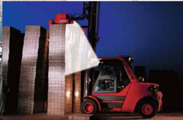
Upper reflector offers a concentrated illumination of the high rise rack
